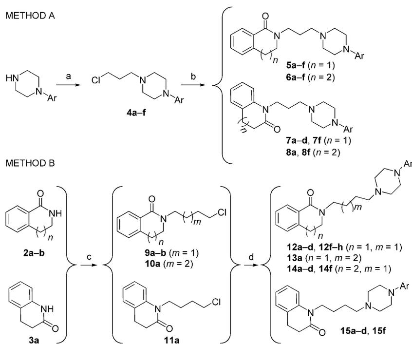
**Scheme 2.** Synthesis of *N*-(arylalkyl)benzolactams. Reagents and conditions: a) 1-bromo-3-chloropropane, NaOH, acetone; b) **2** or **3**, NaH, benzene, reflux; c) 1-bromo-4-chlorobutane or 1-bromo-5-chloropentane, NaH, benzene, reflux; d) arylpiperazine, K<sub>2</sub>CO<sub>3</sub>, KI, methyl isobutylketone, reflux.
